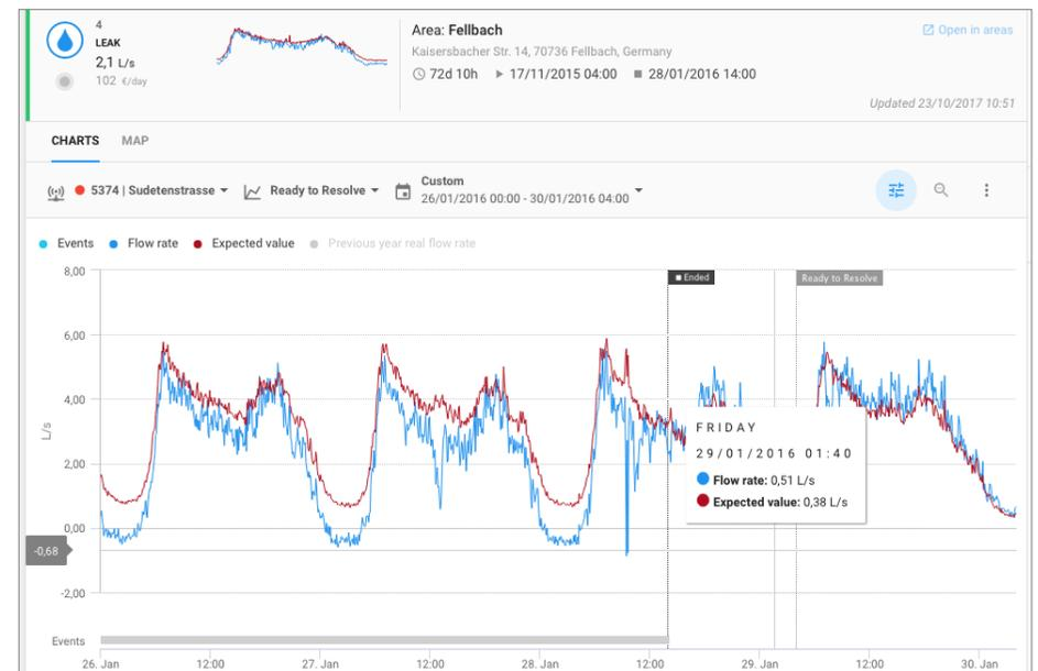
AI and hydraulic simulation provided accurate pre-location of the leak in the supply network.
